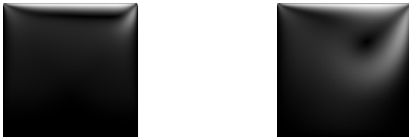
Figure 2.1: Velocity field of a 104x104 2D lid cavity simulation, at iterations 150 (left) and 1000 (right)
